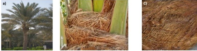
Fig. 1. Photograph of a) date palm tree b) stems surrounding by fibre c) fibres [24]
