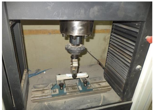
Fig. 4 .Drawing of three-point bending test a) load set up, b) specimen .
